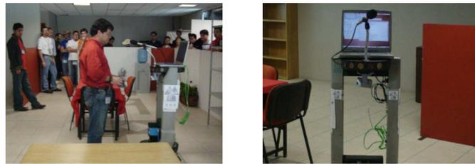
Fig. 9. Markovito learning to recognize an object (left) and later searching for it (right).
