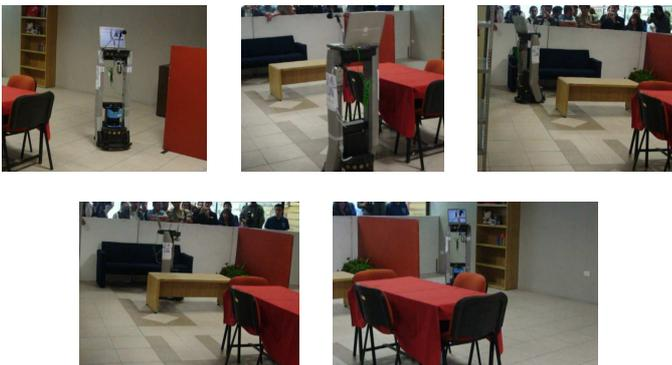
Fig. 8. Markovito navigating through the environment reaching different destination points.
